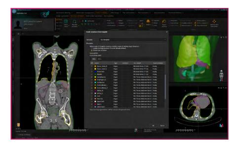
RayDeformable include deformable fusion tools for multimodal images with 2 different GPU-based algorithms, Adaptive and dose accumulation tools
